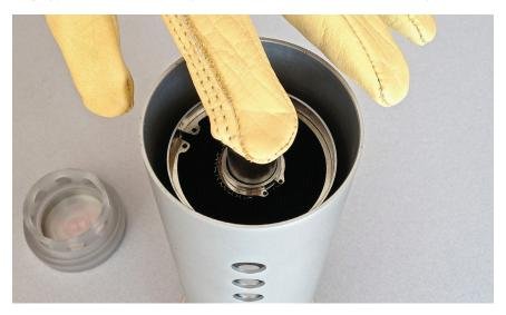
6. You are now ready to reassemble the unit. Insert the top cap into the aluminum body so that the screw holes in the aluminum line up with the threaded holes in the top cap. Reinsert the screws and plug in the power supply. If your air purifier functions normally again, your lamp replacement has been successful.
