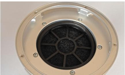
1. Unplug the power supply to the air purifier. Turn the air purifier upside down and set it down on a solid surface. You may want to set it on a paper towel or soft cloth to prevent scratching of the chrome top cap. You will now see the bottom of the purifier, which shows a filter held in place by a rubber o-ring. The rubber o-ring can easily be removed with your fingers, and the old filter cartridge can easily be pulled out.
